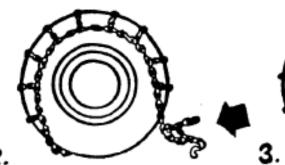
Lay chain over the tyre, cross chain hooks up and the Lever fastener on the outside of the tyre. Tuck the spare length of chain under the tyre.
