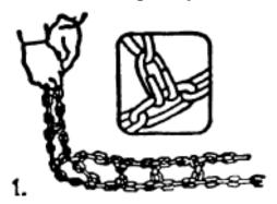
Lay chains out flat, remove all tangles. When chains are placed on the tyre, the cross hook eyes must face up (see the insert). Damage to your tyres could result if these hooks face against the tyre.
